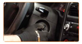
Pull the windscreen wiper stalk to the downward position. By doing so, you will switch the windscreen wipers from the service mode to the operation mode.
