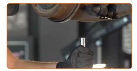
Clean the brake drum. Use a wire brush. Treat the contacting surface. Use copper grease.
