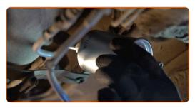
Tighten the fuel filter fasteners. Use Torx T20.
