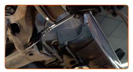
Raise the hydraulic transmission jack by 10-15 cm. Use a hydraulic transmission jack.
