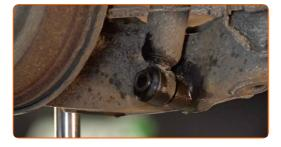
Unscrew the upper fastener of the shock absorber. Use a drive socket #E20. Use a tap wrench.
