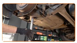
Unscrew the lower fastener of the shock absorber. Use a drive socket #E20. Use a tap wrench.
