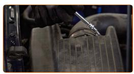
5 Disconnect the air intake pipe from the air filter housing.
