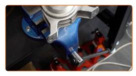
Clean the mounting seat of the engine mount. Use WD-40 spray.
