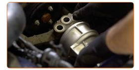
Screw in the engine mount fasteners (6 pieces). Use a drive socket #E20. Use a torque wrench. Tighten it to 55 Nm torque.
