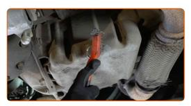
Unscrew the drain plug. Use Torx T40. Use a ratchet wrench.
