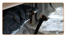
Replacement: engine oil and filter – OPEL ASTRA G Convertible (F67).
