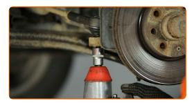
Tighten the tie rod end locknut. Use a combination spanner #22. Use a torque wrench. Tighten it to 60 nm torque.
