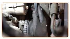
6 Return the tensioner pulley to its initial position.
