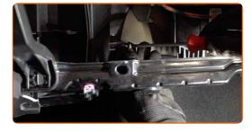
17 Install the air duct housing.
