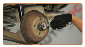
9 Remove the brake drum.
