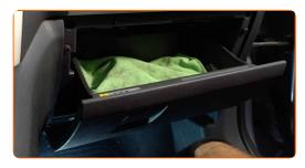
Unscrew the glove box fastening screws. Use Torx T20.
