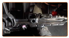
17 Install the air duct housing.
