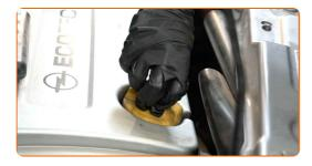
Tighten the oil filler cap.
