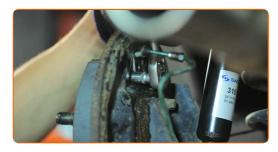
Attach the brake pipe. Use a flare nut spanner #10.
