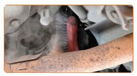
5 Detach the oxygen sensor connector.
