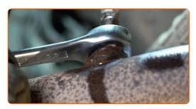
Remove the oxygen sensor.
