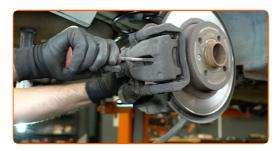
10 Remove the brake caliper.
