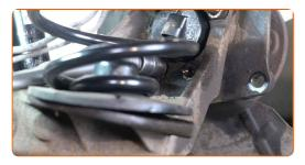
Unscrew the fastener of the ABS wiring harness bracket. Use a drive socket #E8. Use a ratchet wrench.
