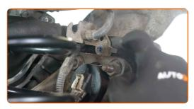
Tighten the fastener of the ABS wiring harness bracket. Use a drive socket #E8. Use a torque wrench. Tighten it to 7 nm torque.
