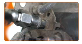
Connect the ABS sensor wiring.
