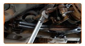
Tighten the fastening nut connecting the tie rod end to the steering knuckle. Use a drive socket #18. Use a torque wrench. Tighten it to 50 nm torque.
