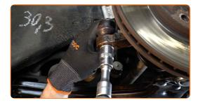
Screw on the tie rod end jam nut. Use a combination spanner #22.
