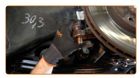
Screw on the fastening nut that connects the tie rod end to the steering knuckle. Use a drive socket #18. Use a ratchet wrench.
