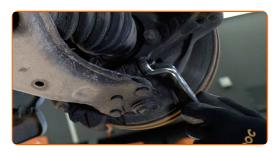
Remove the fastening bolt. Use a hammer. Use a pin punch.
