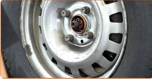
**42** Lower the car and working in a cross order, tighten the wheel bolts. Use wheel impact socket #17. Use a torque wrench. Tighten it to 110 Nm torque.
