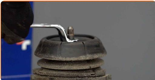
**20** Remove the shock absorber mount, boot and bump stop.
