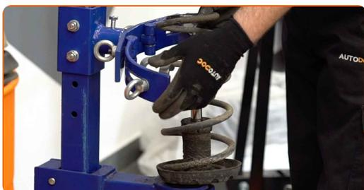
**23** Install the spring on the shock absorber.
