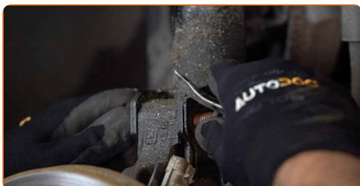
**13** Disconnect the brake hose holder from the shock absorber strut. Use a crowbar.
