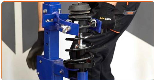
**28** Remove the assembled shock strut.
