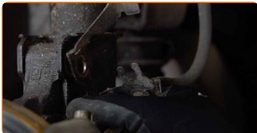
**14** Disconnect the steering knuckle from the shock absorber strut.
