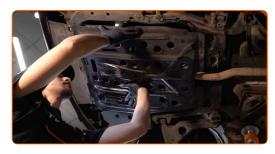
Tighten the fasteners of the oil pan lower cover. Use a drive socket #12. Use a ratchet wrench.
