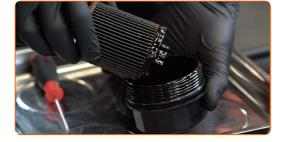
Remove the oil filter cover O-ring. Use a flat screwdriver.
