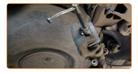
21 Install the brake caliper and fix it.
