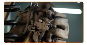
Unscrew the brake caliper fastening. Use a combination spanner #13.
