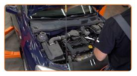
12 Screw new spark plugs and tighten them. Use the spark plug socket #16. Use a torque wrench. Tighten it to 24 nm torque.
