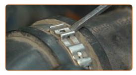
Remove the mass air flow sensor.
