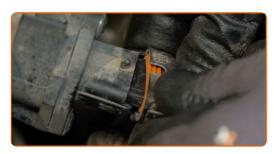
Loosen the fastening clamp connecting the air duct to the air filter housing. Use a Phillips screwdriver.
