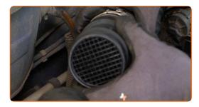
9 Attach the air duct.
