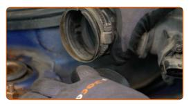
6 Unfasten the clamps that secure the mass air flow sensor to the air hoses. Use a flat screwdriver.
