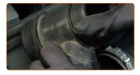
Install a new mass air flow sensor.
