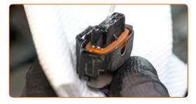
13 Attach the mass air flow sensor connector.
