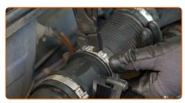
Screw the fastening clamp connecting the air duct to the air filter housing. Use a Phillips screwdriver.
