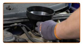
Pour coolant in the coolant reservoir.
