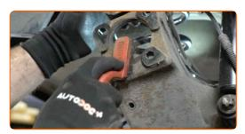
Detach the hub bearing from the brake disc protection plate. Use a hammer.
