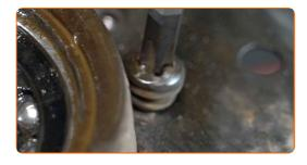
Remove the brake disc cover.
