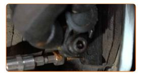
Tighten the fastener that connects the ABS sensor to the steering knuckle. Use HEX No.H5. Use a torque wrench. Tighten it to 8 Nm torque.
