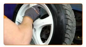
Unscrew the fastener connecting the drive shaft to the wheel hub. Use a drive socket #30. Use a ratchet wrench.
