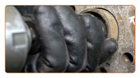
Remove the wheel bearing washer. Use a crowbar.
