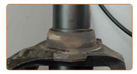
Press out the inner bearing race that is remaining on the hub. Use a bearing separator.
