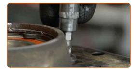
Clean the wheel hub mounting seat. Use all-purpose cleaning spray.
