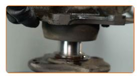
Clean the mounting seats of the shock strut. Clean the mounting seat of the tie rod end. Clean the splines of the drive shaft CV joint. Clean the ball joint mounting seat. Use a wire brush. Use WD-40 spray. Use copper grease.
