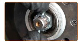
Install the cap of the hub nut. Use a rubber mallet.
