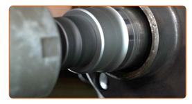
Clean the hub. Use a wire brush. Treat the contacting surface. Use ceramic grease.
