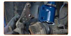
Detach the driveshaft from the steering knuckle.
