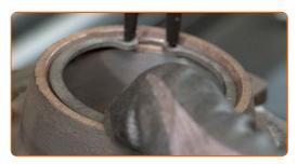
Press-fit the new bearing into the steering knuckle. Use a bush and bearing driver set.
