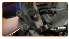
Clean the wheel hub bearing retaining ring. Use a wire brush. Use WD-40 spray.
