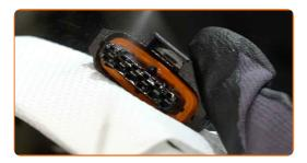
Plug in the ignition coil connector.
