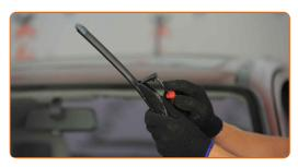
Remove the blade from the wiper arm.
