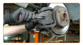
10 Remove the brake caliper.
