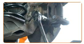
Remove the caliper bracket.
