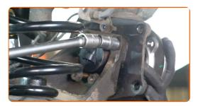
Tighten the hub bearing nuts. Use a drive socket #16. Use a torque wrench. Tighten it to 50 Nm torque.+45°
