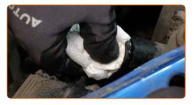
Clean the thermostat housing. Use a wire brush. Use all-purpose cleaning spray.
