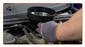
Pour coolant in the coolant reservoir.
