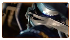
Remove the fuel filter. Put the old filter cartridge in the container.
