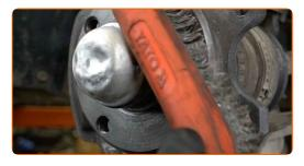
20 Install the brake disc.
