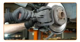
10 Remove the brake caliper.
