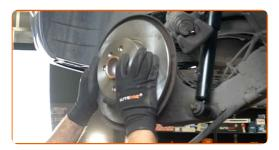
Tighten the brake disc fastening. Use Torx T30. Use a torque wrench. Tighten it to 8 nm torque.
