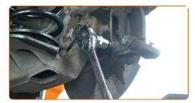
14 Remove the caliper bracket.
