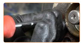
Remove the brake disc.
