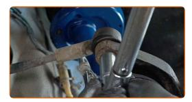
Tighten the lower fasteners of the suspension strut. Use a drive socket #18. Use a torque wrench. Tighten it to 90 Nm torque.+45°
