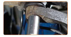
Screw the fastener connecting the ball joint to the steering knuckle. Use a combination spanner #13. Use a drive socket #13. Use a ratchet wrench.
