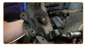
Clean the wheel hub bearing retaining ring. Use a wire brush. Use WD-40 spray.
