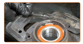
Tighten the fasteners of the brake disc back plate. Use a Phillips screwdriver. Use a torque wrench. Tighten it to 7 Nm torque.
