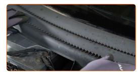
Install and secure the cowl grille. Use a drive socket #8. Use a ratchet wrench. Use a Phillips screwdriver.
