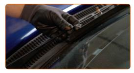
Tighten the wiper arm fasteners. Use a drive socket #13. Use a torque wrench. Tighten it to 14 Nm torque.
