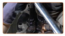
16 Remove the caliper bracket.
