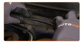
Remove the fender protection cover.
