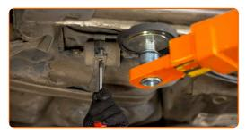
Squeeze the clips and detach the fuel supply lines from the fuel filter housing. Use fuel line pliers.
