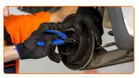
15 Remove the brake pads.
