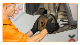
Tighten the hub. Use a drive socket #27. Use a torque wrench. Tighten it to 175 nm torque.
