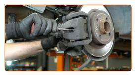
10 Remove the brake caliper.
