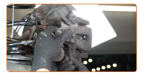
Install the parking brake cable into the brake caliper bracket. Use water pump pliers. Use a crowbar.
