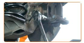
14 Remove the caliper bracket.
