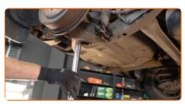
Unscrew the lower fastener of the shock absorber. Use a drive socket #E20. Use a tap wrench.
