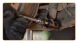
Remove the fastening bolt.
