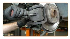
11 Remove the brake caliper.
