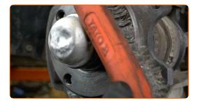
20 Install the brake disc.
