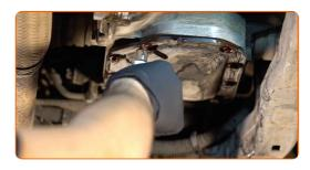
10 Remove the transmission fluid pan.
