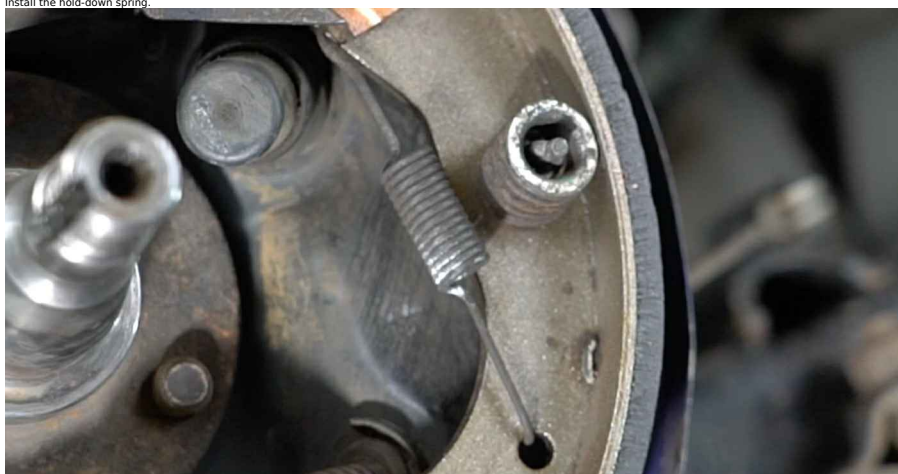
40 Install the upper return spring. Use long nose pliers.
