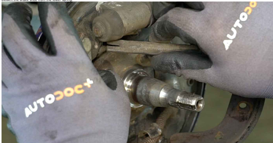
18 Remove the right brake shoe.
