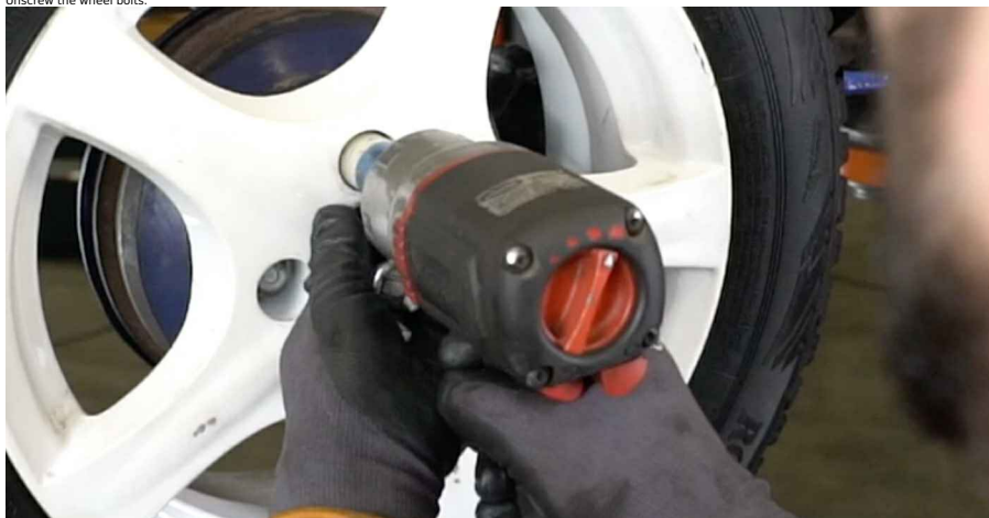
50 Unscrew the wheel bolts.
