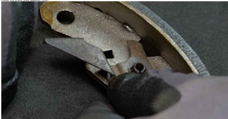
34 Install the circlip.
