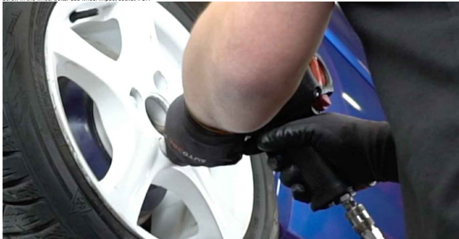
47 Screw in the wheel bolts. Use wheel impact socket #17.
