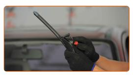
Remove the blade from the wiper arm.
