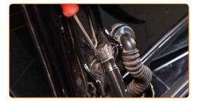
Release the circlip connecting the gas strut to the car body. Use a flat screwdriver.
