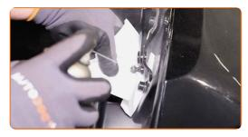
Install the new boot lid gas strut.
