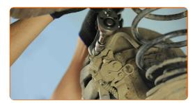
Treat the surface where the brake disc contacts the wheel rim. Use high-temperature ceramic grease.
