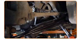
Use a combination spanner #19. Use a drive socket #18. Use a torque wrench. Tighten it to 65 Nm torque.
