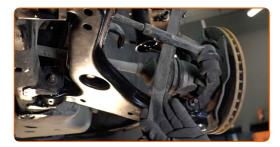
11.1 Install a new rod, tighten the fasteners.
